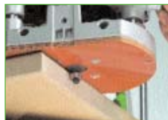
Simply fit it: tool-free change between base runner and copying ring (also available for jointing system VS 600).
